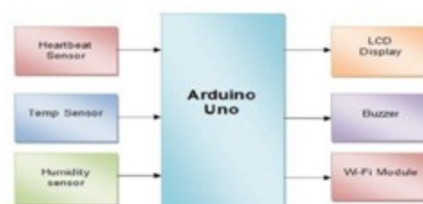
Block Digram of IOT based health care monitoring system
