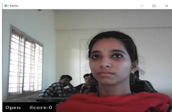
Figure.5.1 input and scoring when the state of eye is open.
