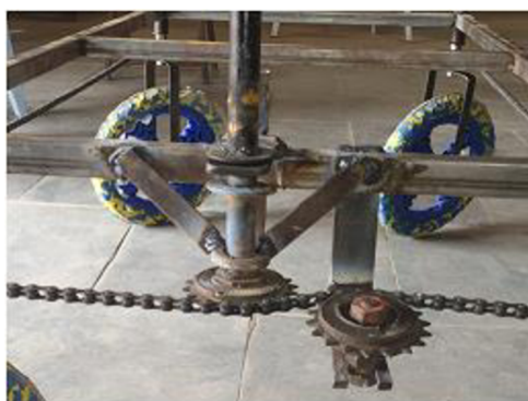
Fig 5: The arrangement of steering wheel with gears
