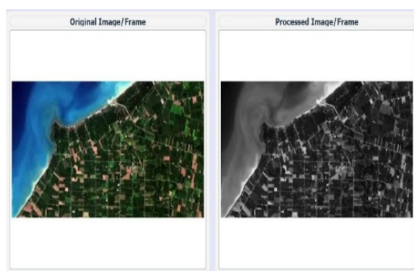
Fig.3 Visualization of grayscale conversion applied to an image
