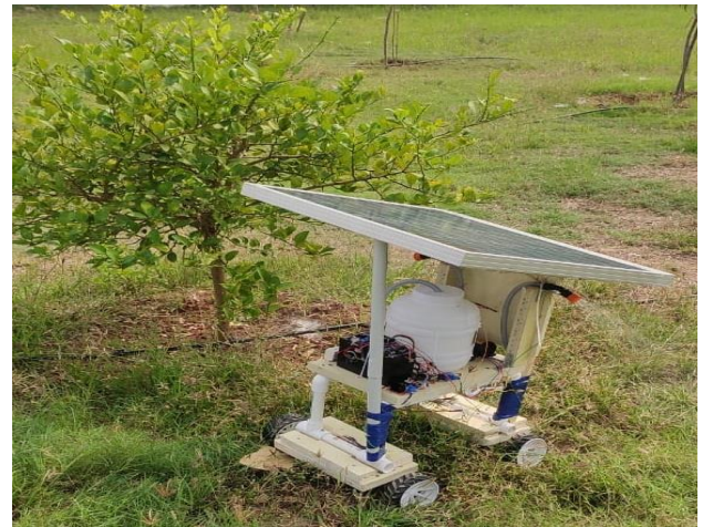
Fig.9 Developed model of Solar Powered Electric Vehicle mounted Pesticide Sprayer
