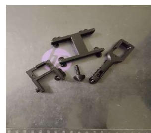
Figure.11 3D Printed Coxa, Femur and tibia
