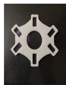
Figure.10 3D Printed Upper frame of Hexapod
