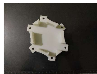
Figure.9 3D Printed Base of Hexapod
